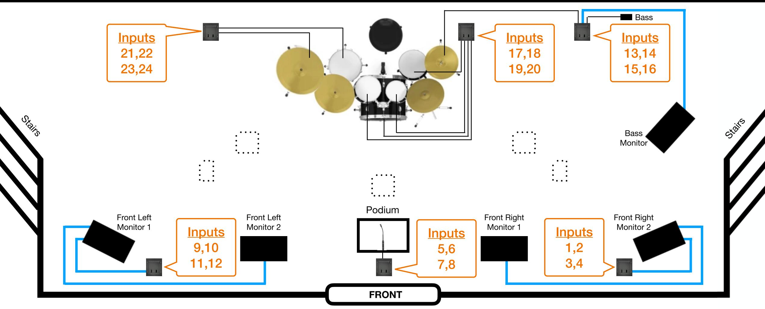
As of 02-14-2023, all stage pocket XLR & Speak-On connectors have been replaced & are fully usable. As of 02-14-2023, the (7) drum microphones have been relocated to free up two inputs back L & two back R. Dotted line boxes pictured are very old stage pockets that are no longer used.
