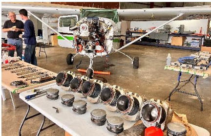
Preparing to install 6 cylinders on the C182
