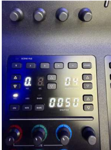
MASTER GAIN display and up/down arrow buttons.
