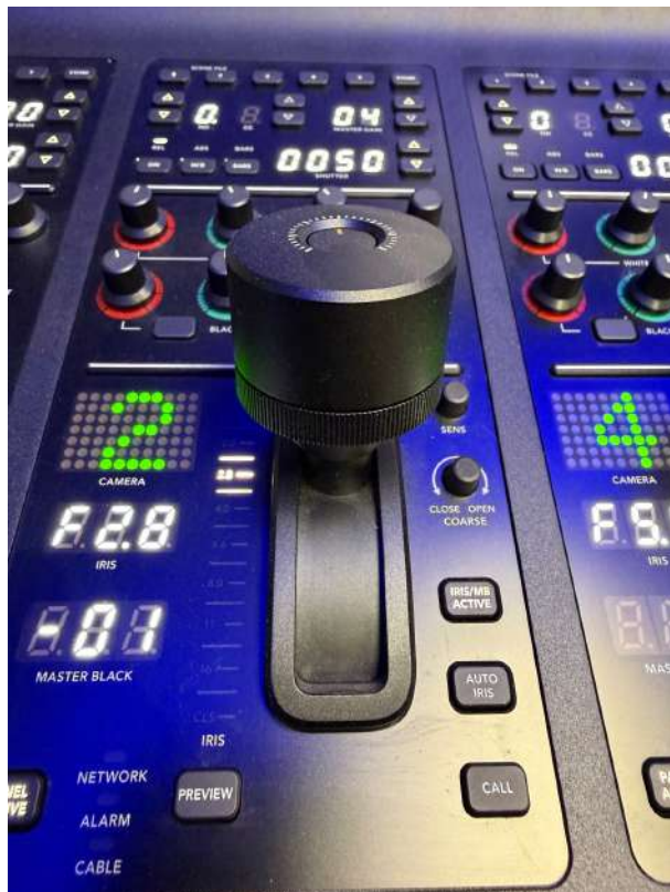
Left: large iris knob and travel slot. Right: iris readout and PANEL ACTIVE status.
