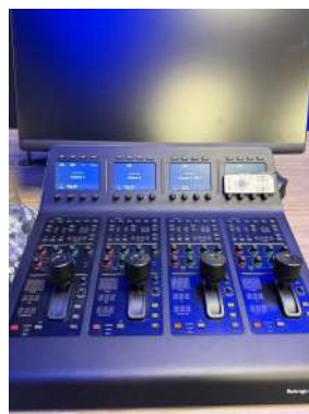
Inactive state: the PANEL ACTIVE button on each section is red.
