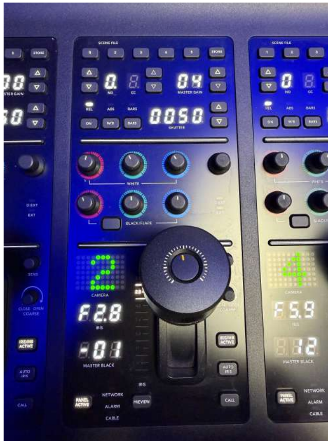
A single camera section showing the camera number, iris controls, and exposure controls.
