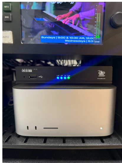
Healthy XDIP status example: LNK, USB, VID, and PWR indicators are illuminated.
